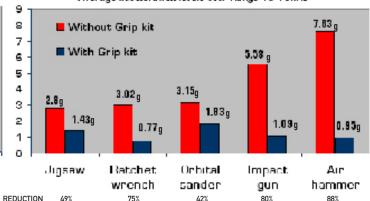
Test show average vibration reductions in a variety of hand tools after a Grip kit has been applied. Results obtained using Bruel & kjar Vibration Meter. Model 2516, for comparison only. Individual test results may vary according to hand size, grip strength, age and manufacturer of tool and other environmental factors.
